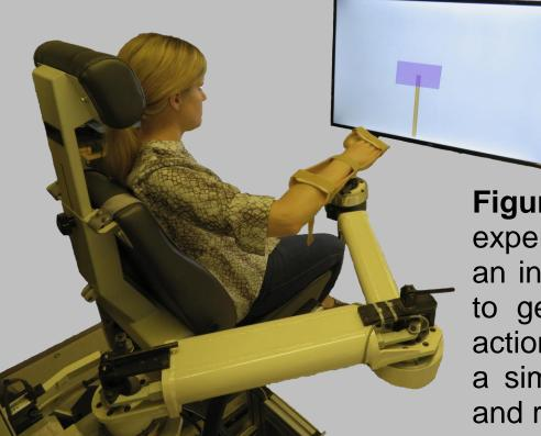
Figure 1B: Upper limb robotic platform used during experiments. It provides haptic feedback to simulate an inertial model via admittance control and is able to generate enough force to overpower a user's actions. In our experiments we asked users to invert a simulated cart-pendulum system, providing input and receiving guidance through the robot.
