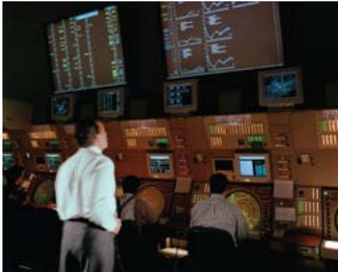
CTAS provides automation tools for air traffic controllers to use in planning and controlling arrival traffic. It includes methods for achieving acceptable aircraft sequencing and separation as well as improved airport capacity. This photo shows CTAS' Traffic Management Advisor (TMA) in operation in the Denver airport facility. FAA operates TMA at all of its centers and says it has fundamentally changed National Airspace System (NAS) operations.
