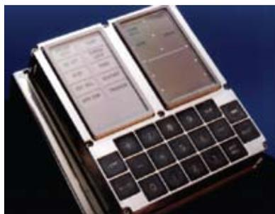
Apollo computer interface box used in the F-8C digital fly-by-wire program.
