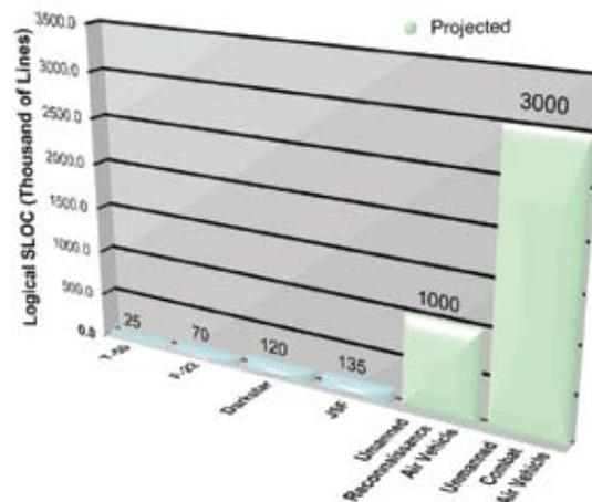
Complexity growth, as measured by logical software lines of code, of future safety-critical flight control systems (autonomy)
