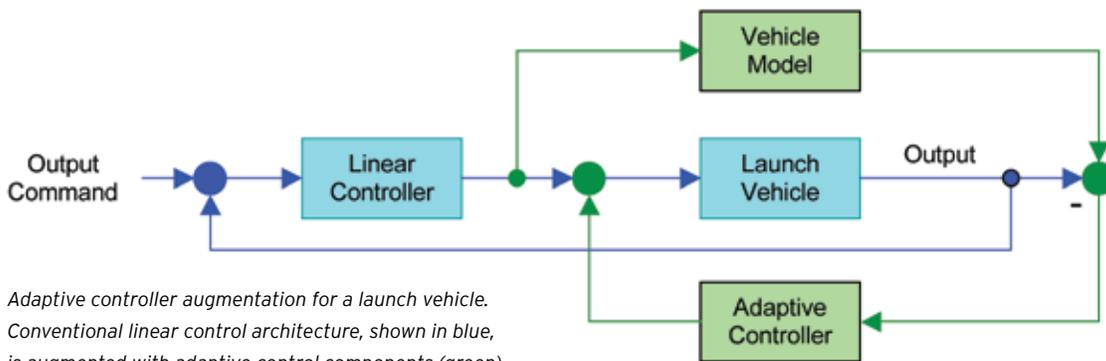
Adaptive controller augmentation for a launch vehicle. Conventional linear control architecture, shown in blue, is augmented with adaptive control components (green).
