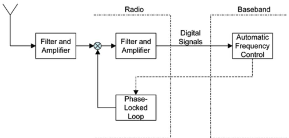
*Mobile phones include a radio unit, which works with analog signals at high frequencies using analog circuits, and a baseband unit, which works with digital signals using digital hardware blocks and special-purpose digital signal processors. Automatic frequency control thus controls the analog phase-locked loop using digital symbols.*
