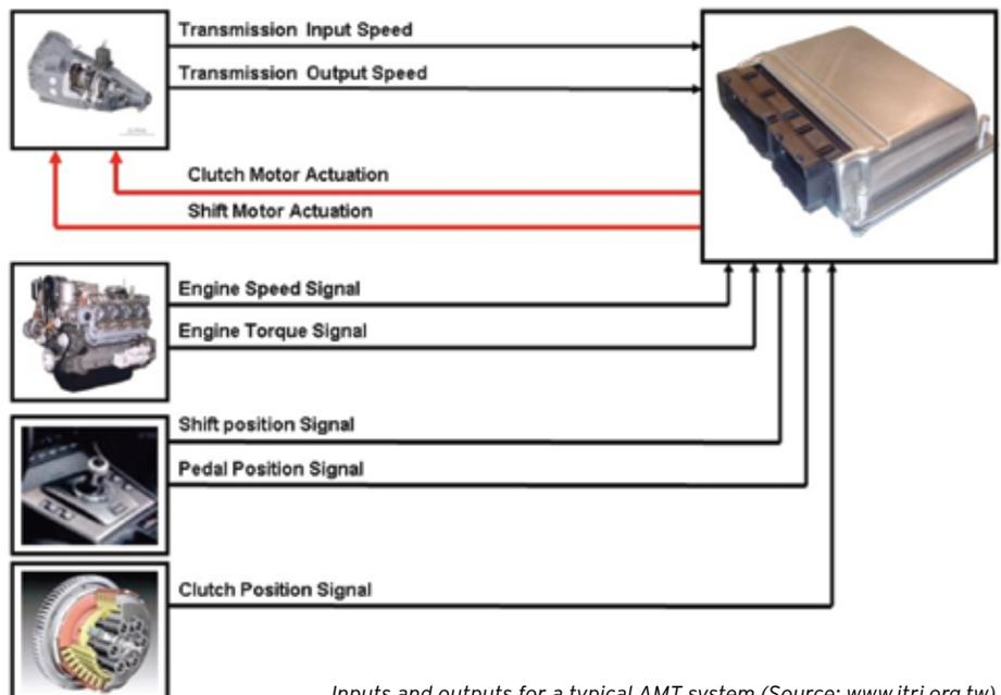
Inputs and outputs for a typical AMT system (Source: [www.itri.org.tw](http://www.itri.org.tw))
