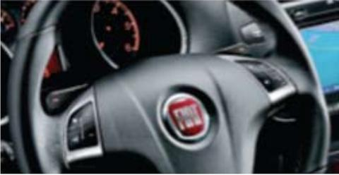
Shift buttons on the steering wheel of a FIAT Bravo
