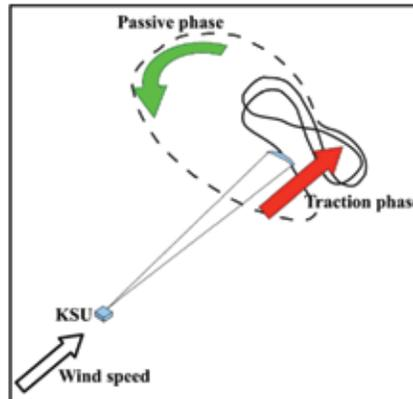
One example is a technology developed at Politecnico di Torino called the “Kitenergy” system. The concept is based on wings (for example, power kites like the ones used for surfing or sailing) linked to a kite steering unit (KSU) on the ground. Two lines serve both to control the kite’s flight and to convert the aerodynamic forces into electrical power by using suitable rotating mechanisms and electric drives kept on the ground. In one
