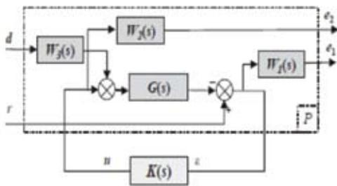
Figure 2: Standard four-block  $H_\infty$  scheme.
