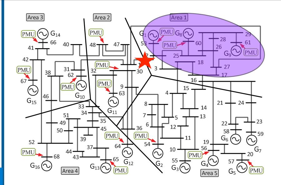
Disturbances lead to oscillations in voltage/current phase and frequency
