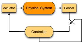
Constant monitoring of the state is no longer needed although the loop is still closed based on the current performance.
