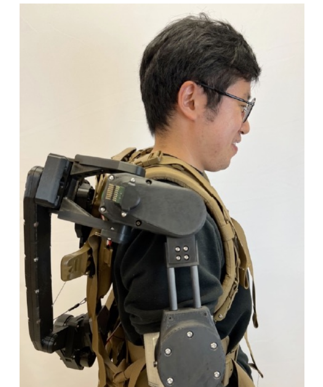
Wearable upper-extremity exoskeleton robot with a hybrid actuation mechanism.
