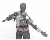
Illustration of the wearable upper-extremit exoskeleton robot with a hybrid (parallel and serial) actuation mechanism
