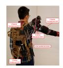
Initial prototype of the wearable upperextremity exoskeleton robot with a *hybrid* (parallel and serial) actuation mechanism.
