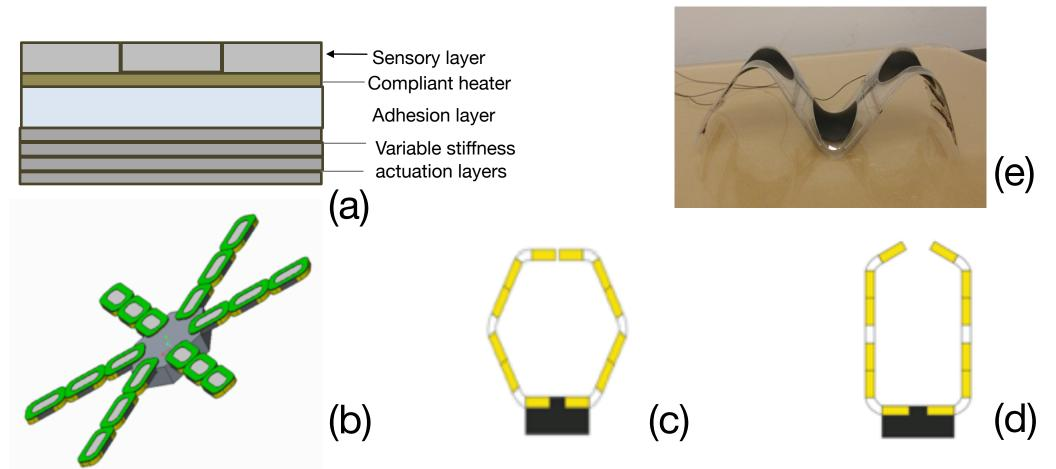
(a) Cross-section of an individual finger (b) 3D model of 18 rotary joint actuator. (c) Illustrations of deformed structure showing two 3-joint actuators iterated together to form a closed grip. (d) The same actuators could an also maintain a small gap (e) A multi-segmented actuator is shown contorting its conformation
