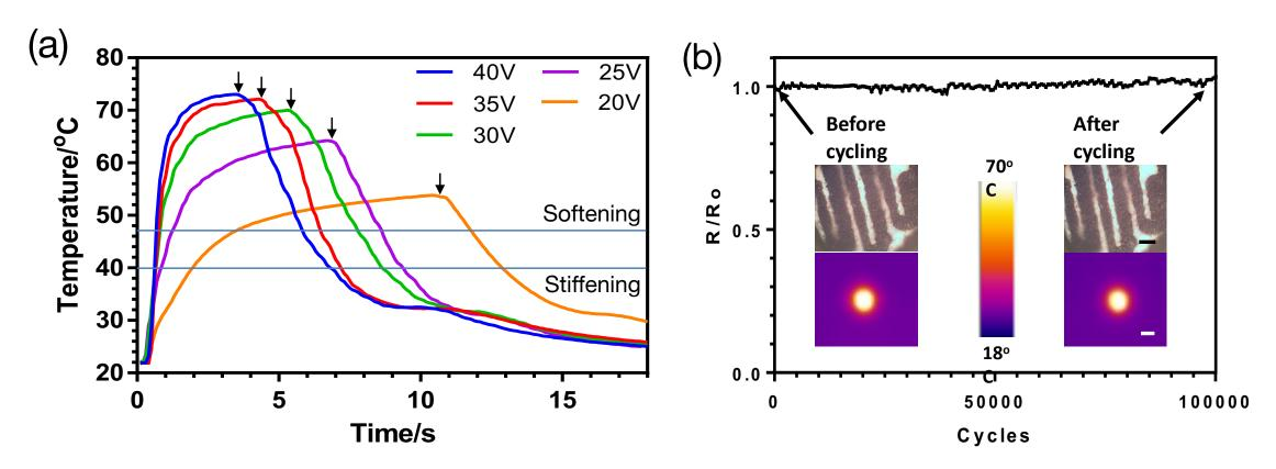
(a) Temperature profiles of serpentine-CNT electrode under different voltage supplied. As the voltage increases, the heating rate increases (b) Lifetime cyclic testing with 100% area expansion
